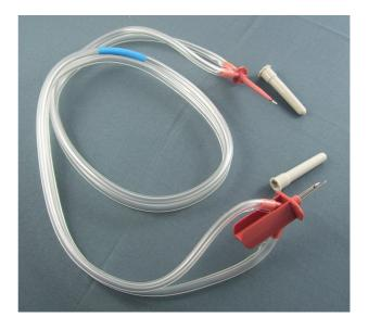
Pic. 1 SVP Dilutor : Tubing with Needle Connections
